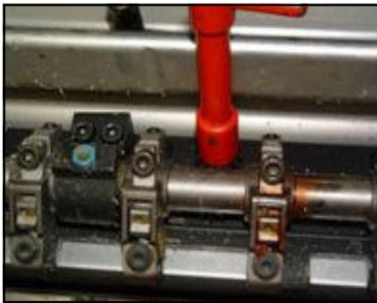
Rotate the cylinder so the gripper end is exposed. Open the slot just below the grippers by loosening the unlocking bolt. Clean out the slot with a flat piece of metal to ensure no debris is obstructing the slot.
