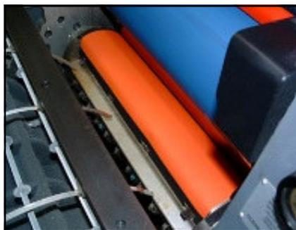
Rotate transfer cylinder and inspect for a good tight fit all around the cylinder. Verify the jacket is properly installed before running the press.
