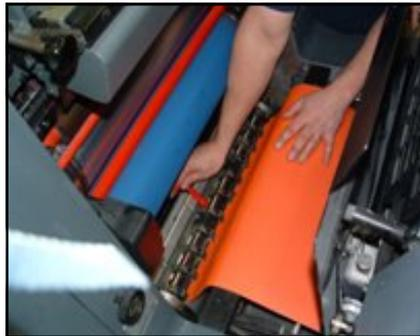
Ensure the jacket is centered on the cylinder and the leading edge of the SS strip is **uniformly below** the cylinder level and then tighten down the lockdown bolt.
