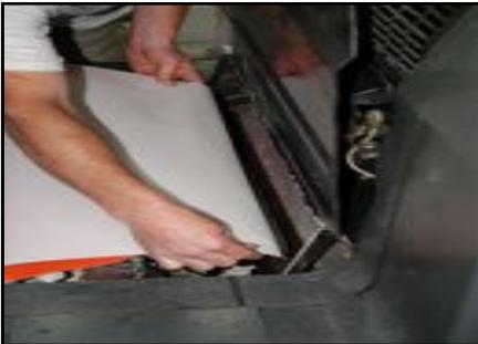
Loop the jacket and lay onto the cylinder. Gently insert the stainless steel flat strip into the slot (centering the jacket on your press cylinder).
