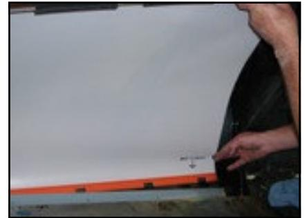
Install the **Non-elastic** Orange diecut side of the **Orange** Jacket first (this jacket side is marked with a black arrow and the words "Install this side first"). Rotate the cylinder back to a position where you have hand accessibility to the pin-like bolt heads on the gripper end. Turn off the press.
