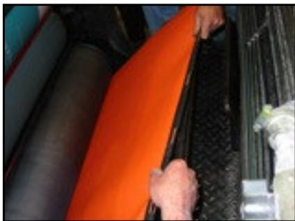
Pick up the jacket by the black elastic loops/steel rod, and slowly rotate the cylinder (continually feeding the jacket so that it wraps the cylinder in a tight and square/true manner) until you have access the pin holes on the transfer cylinder plate. Turn off the press.
