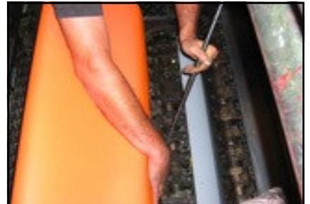
Carefully lay the Black elastic side of the Orange Jacket Orange side up so it droops over the open access cover (that you open to expose the transfer cylinder). Snap the steel rod behind each pin-like bolt head, further ensuring that the steel rod is secured under the locking spring. You can usually hear an audible click. Center the jacket on the cylinder also ensuring the pin-like bolt heads are in the center of the die cut areas. *Make sure steel rod is also centered on press.*
