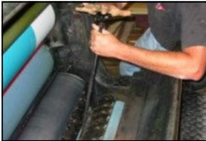
Rotate the transfer cylinder until fully exposing the pin-like bolt heads which secure the steel rod through the die cut portion of the jacket. Turn off the press. Use the Heidelberg "J" tool or duckbill tool to apply downward force on the steel rod and un-snap the rod from behind the pin-like bolt head. Start at one end and continue un-snapping the steel rod along each die cut portion until finished.
