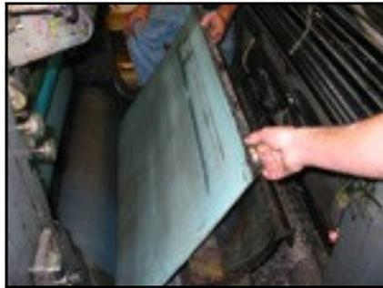
While holding onto the old jacket/steel rod, slowly rotate the cylinder until the gripper end is exposed and the other end of the jacket is exposed. Turn off the press. Reach down with your hand and un-snap the steel rod from behind each pin-like bolt head. Remove the old jacket. **Keep the steel rods for installation.**
