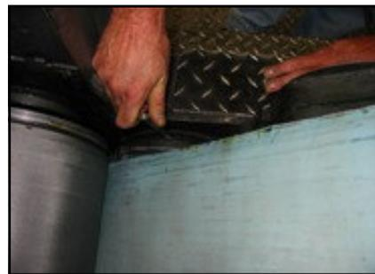
While holding onto the old jacket/steel rod, rotate the cylinder until the lock bolts at both edges of cylinder are accessible with a 17mm wrench to fully loosen.
