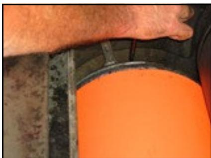
Use the pen like tools to push the cylinder back into its running place (around 1" back, so cylinder lip covers the loops you just installed. You should hear a solid clunk sound letting you know you are fully seated). Now, using the 17mm wrench, tighten down to the lock down bolts on either end of the cylinder. Tighten these bolts securely. Ensure jacket remains centered on cylinder, adjust if necessary.
