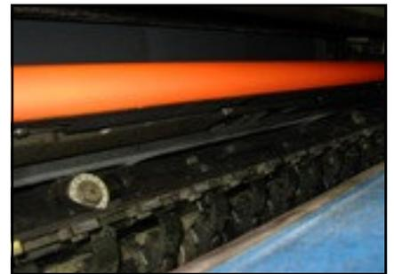
Now, close the flip up portion of the cylinder so that the spring retaining clamp engages. You should feel the jacket tensioning and undergoing slight compression for a perfect fit. Tighten the 13mm lock down bolts on either end of the cylinder.
