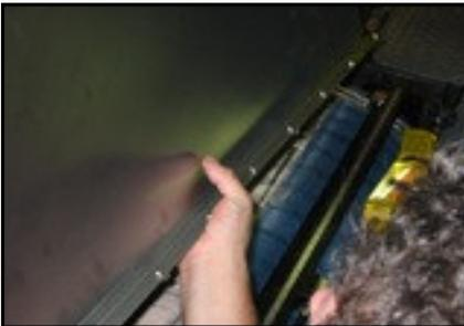
Stop the press when gripper ends emerge. Push out the 10 pins that hold the gripper end of the jacket into the spring bar. Remove jacket.
