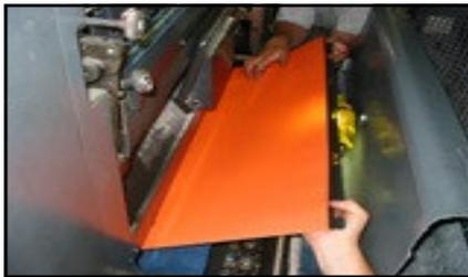
While still holding onto the black elastic/steel rod end of the jacket, rotate the cylinder (continually feeding the jacket so that it wraps the cylinder in a tight and square/true manner) until you come to the flip up portion of the cylinder.
