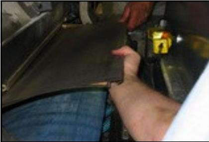
While holding onto the old steel jacket/ Superblue® loop jacket, rotate the cylinder keeping a firm grip on the old jacket and pulling it out.
