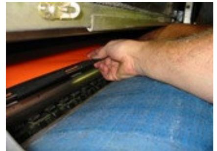
Turn off the press. Unsnap the spring that holds the flip up portion of the cylinder down.
