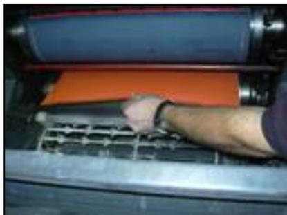
**II. Install new PrintGuardPus<sup>®</sup> Orange glass beaded jacket (No packing Required; the jacket comes pre-packed)**
