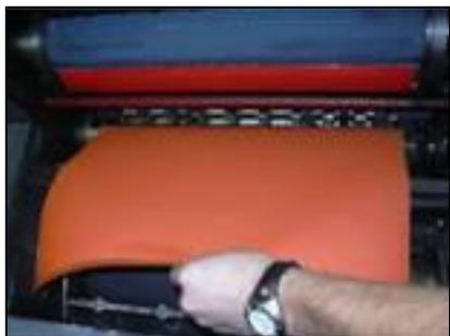
Insert the 3/4" flat stainless steel strip into the pre-opened slot (centering the jacket on your press cylinder). Please ensure the flat
