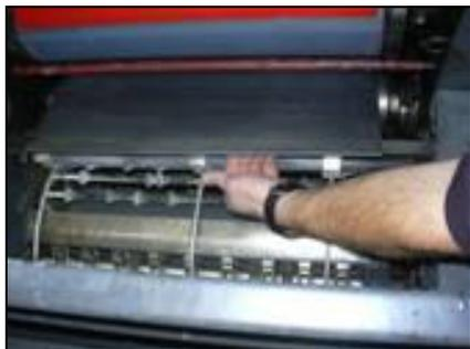
Ensure the jacket is centered on the cylinder and the leading edge of the SS strip is **uniformly below** the cylinder level and then tighten down the 17mm lockdown bolt.
