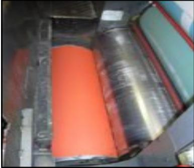
Final inspection: Rotate transfer cylinder and inspect for a good tight fit. Verify the jacket is properly installed and all parts are firmly secured before running the press.
