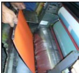
Center the jacket on the cylinder also ensuring the pin-like bolt heads are in the center of the die cut areas.
