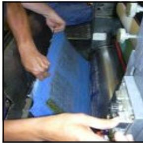
While holding onto the old jacket/steel rod, slowly rotate the cylinder until the gripper end is exposed and the other end of the jacket is exposed. Turn off the press. Reach down with your hand and un-snap the steel rod from behind each pin-like bolt head. Remove the old jacket. Keep the steel rods for installation. Clean the transfer cylinder if necessary.
