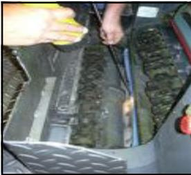
Turn off the press. Use the Heidelberg “J” tool or duckbill tool to apply downward force on the steel rod and un-snap the rod from behind the pin-like bolt head. Start at one end and continue un-snapping the steel rod along each die cut portion until finished.
